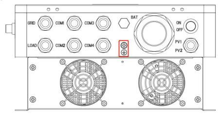
**Note:** As far as possible, the ground cable should be much thicker as possible (the sectional area of wire should not be less than 4mm²) and the grounding point should be kept close to the inverter as possible. The ground wire shall be shorter as possible.
