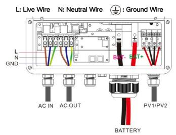
3 Connect the AC output line properly according to the cable sequence and terminal position shown in the above figure. Please connect the ground wire first, then the live wire and the neutral wire.
