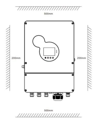
**Step 2:** Open 4 holes in the wall according to the following dimensions, and knock in expansion screws, as shown in the following figure:
